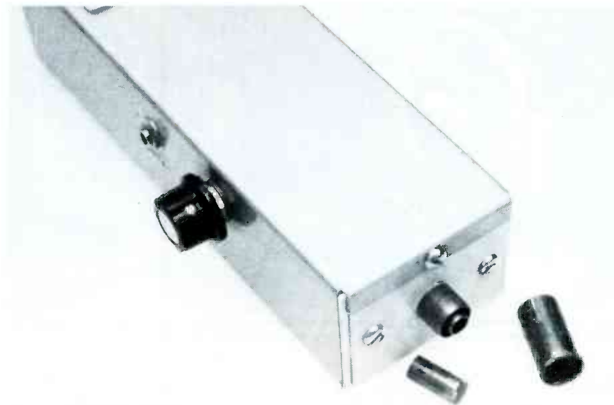
FIG. 8—THE ATTENUATOR'S mounting plate is installed directly over photoresistor Q1. The inner and outer filters are slipped into position when needed.
