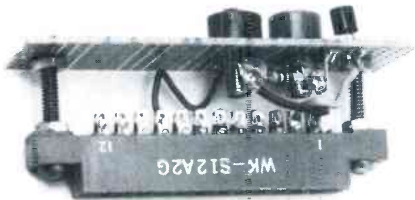
FIG. 2—ALTHOUGH THE LAYOUT ISN'T CRITICAL, try to approximate this layout to insure the interface will fit on the user port.
