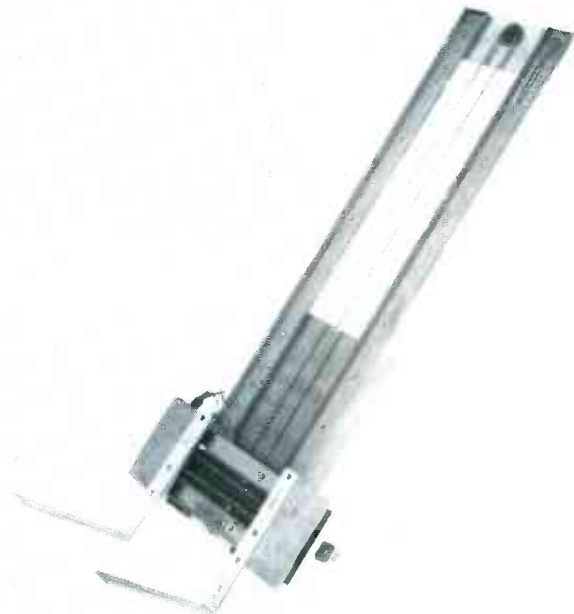
FIG. 1—THIS FORK-LIFT DESIGN can do almost as much as a multi-jointed arm, but with higher lifting capacity and at a lower cost. For greater dexterity, the pincher shown can be added. That pincher, part of which is shown here, will be described in detail in an upcoming installment of this series.
