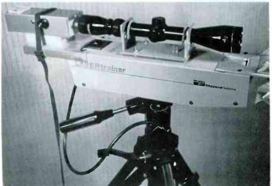
FIG. 2—FOR LONG-RANGE USE the laser and the receiver should be combined into an integral unit so both are aimed together. The telescopic signal provides precision aiming on the target.
